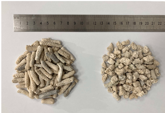
Fig. 1. Photograph of two representative types, namely stick-like and lump-like, of coral sand particles.
